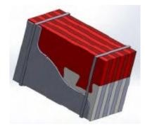
Reduce the cost of your full thickness 1600°C (3000°F) module with FC-Combi Module . A hot face of 1600°C Polycrystalline Fiber, custom cut and matched with a standard RCF blanket cold face. This optimizes the cost structure of the FC-Combi Module by having the Polycrystalline fiber only where it is required.
